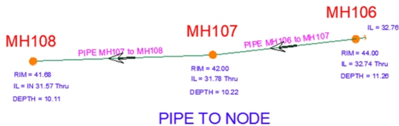
Figure 16 Drainage Pipe Ground and Invert Levels simplified
