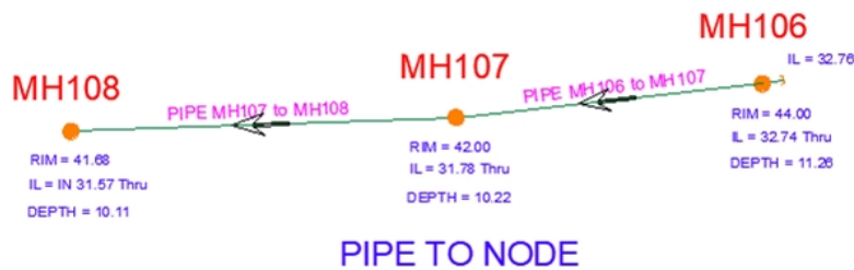
Figure 16 Drainage Pipe Ground and Invert Levels simplified
