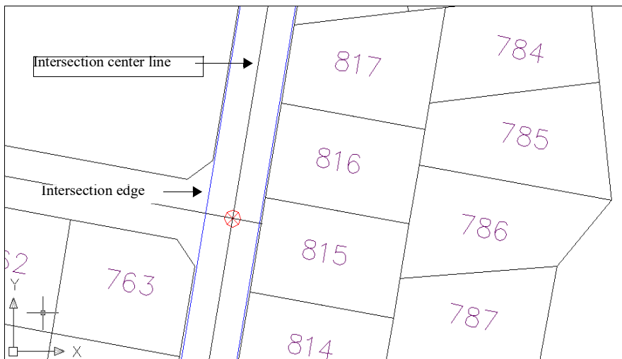
Figure 1 Road intersection center lines and road intersection edges
