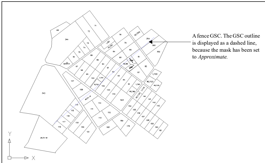
Figure 11 Example of a fence GSC
